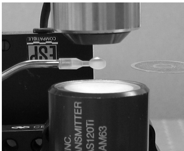
Fig. 2. Image of the bottom excitation configuration of the experimental set-up. The interferometer laser beam is visible on the top of the tablets.
